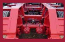
Unique bucket well / boom well configuration provides lowest excavator transport height in the industry.
